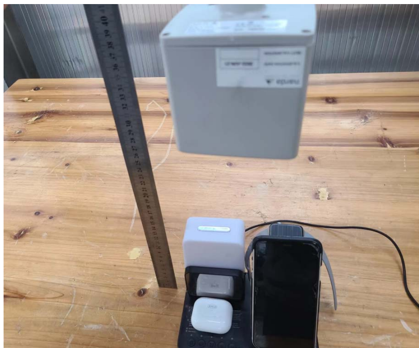
Test Position F-20cm from the edge of EUT to the geometric center of the probe
