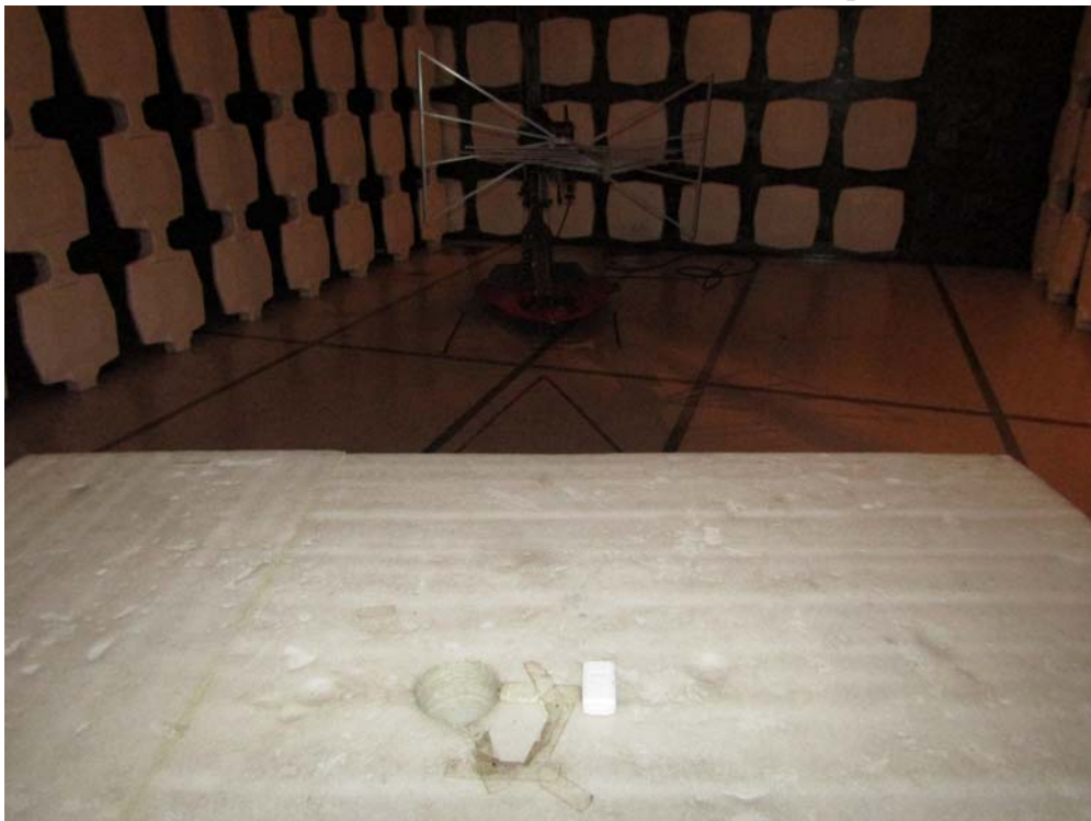
Measurement of Radiated Emission Test Set Up
