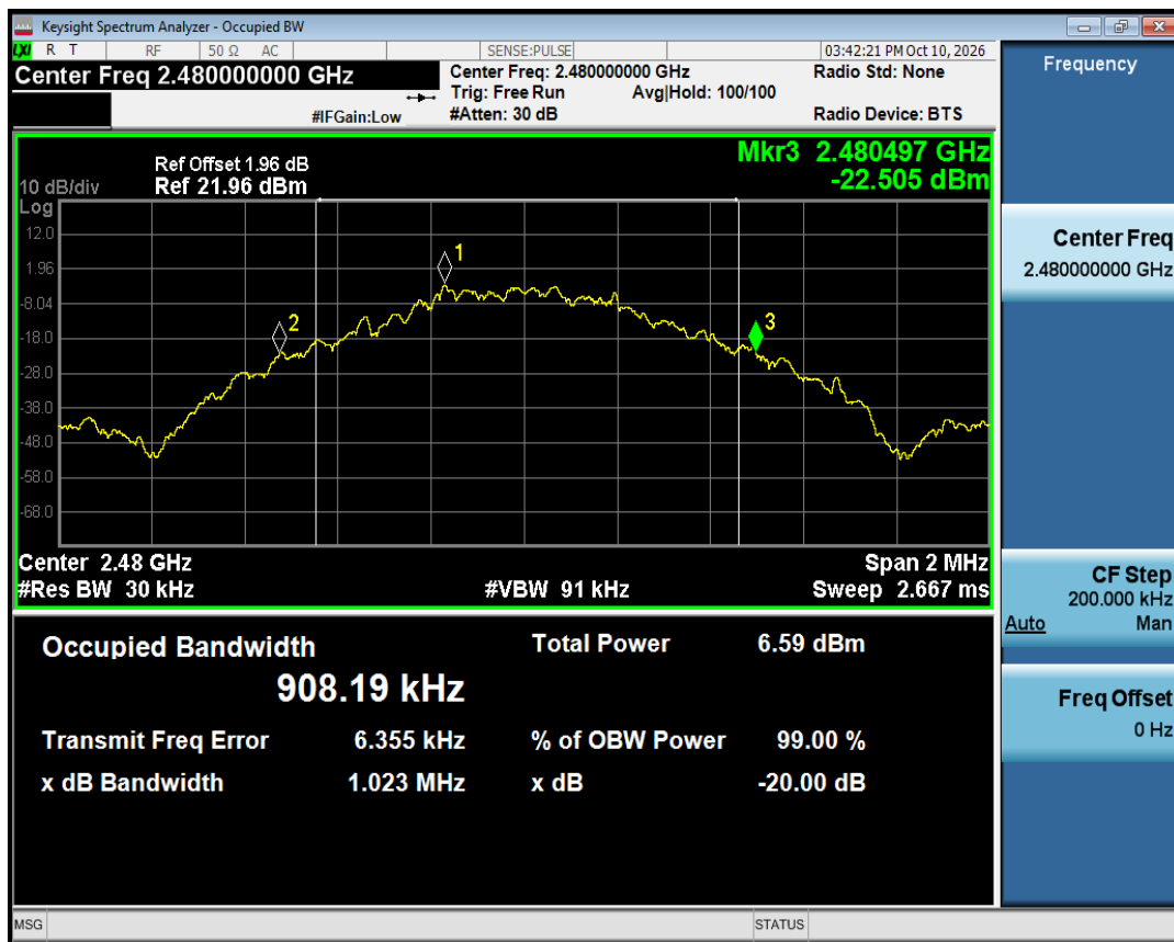
-20dB Bandwidth NVNT 1-DH5 2480MHz Ant1
