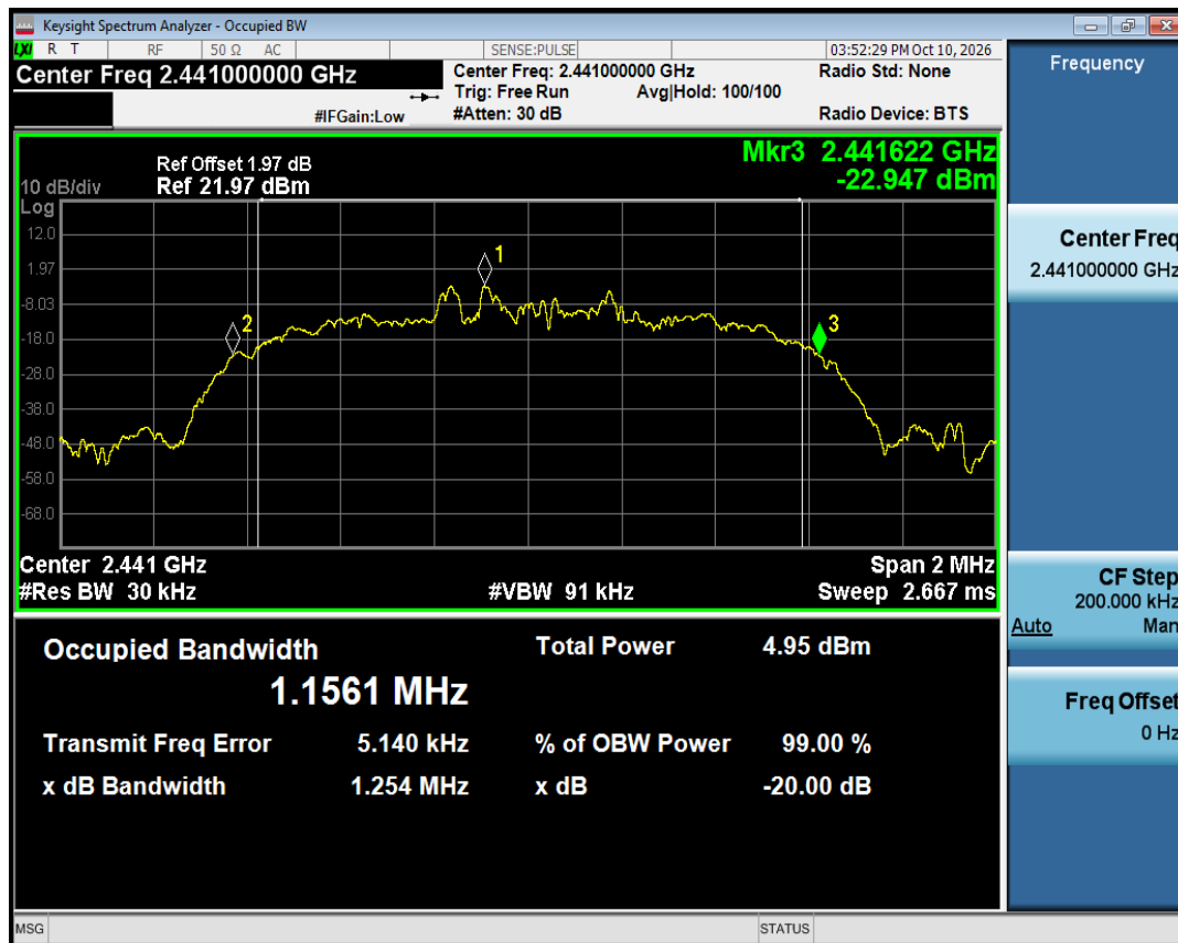
-20dB Bandwidth NVNT 3-DH5 2441MHz Ant1
