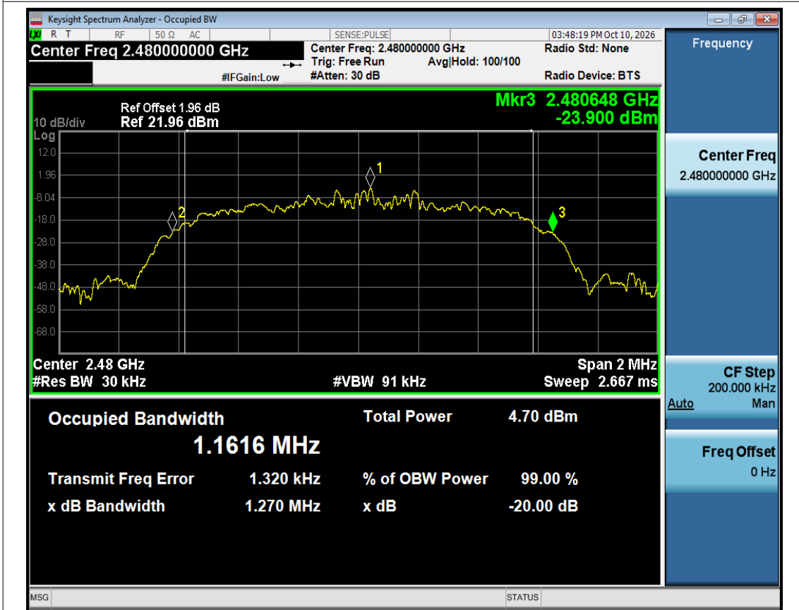
-20dB Bandwidth NVNT 2-DH5 2480MHz Ant1
