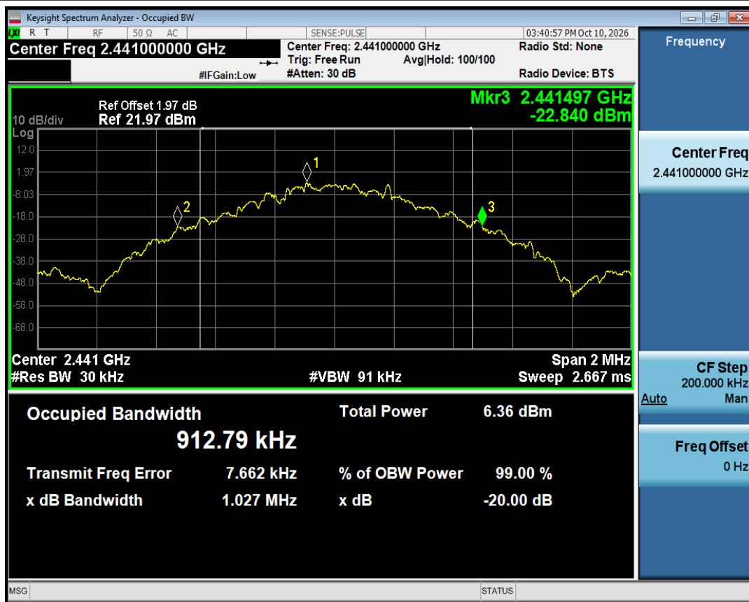
-20dB Bandwidth NVNT 1-DH5 2441MHz Ant1
