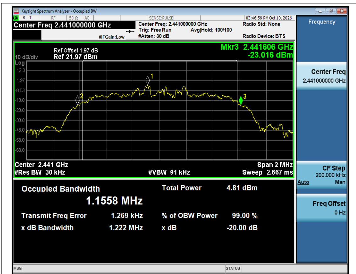
-20dB Bandwidth NVNT 2-DH5 2441MHz Ant1
