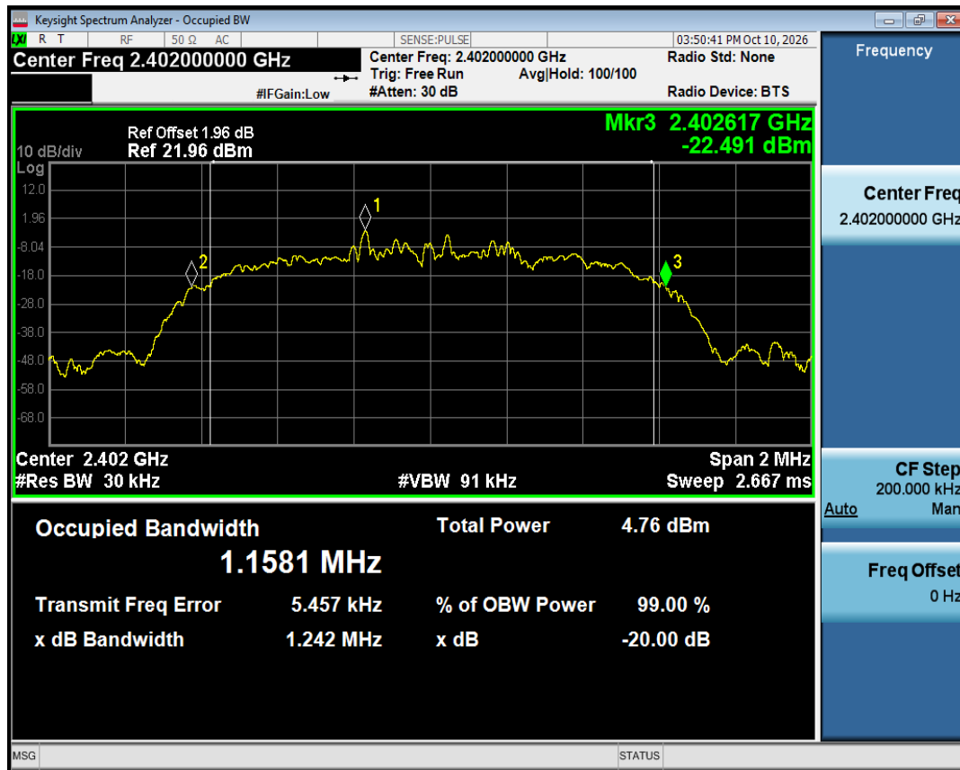
-20dB Bandwidth NVNT 3-DH5 2402MHz Ant1
