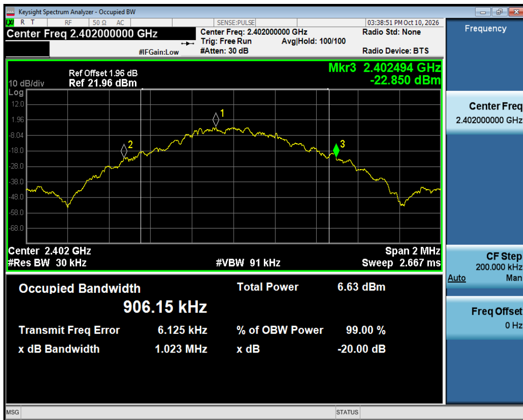
-20dB Bandwidth NVNT 1-DH5 2402MHz Ant1
