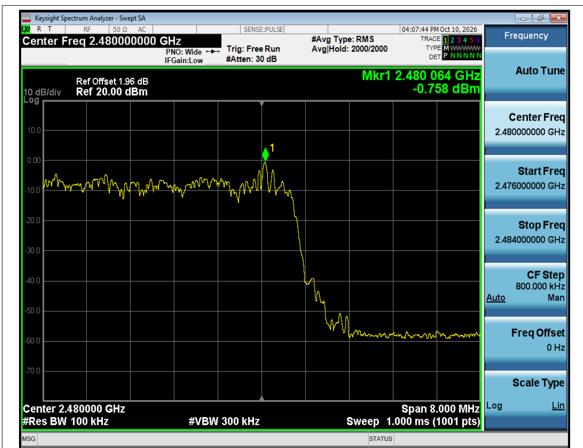
Band Edge(Hopping) NVNT 2-DH5 2480MHz Ant1 Hopping Ref
