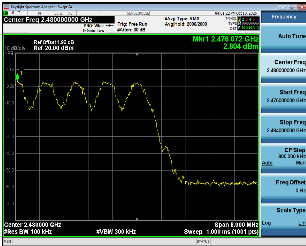
Band Edge(Hopping) NVNT 1-DH5 2480MHz Ant1 Hopping Ref
