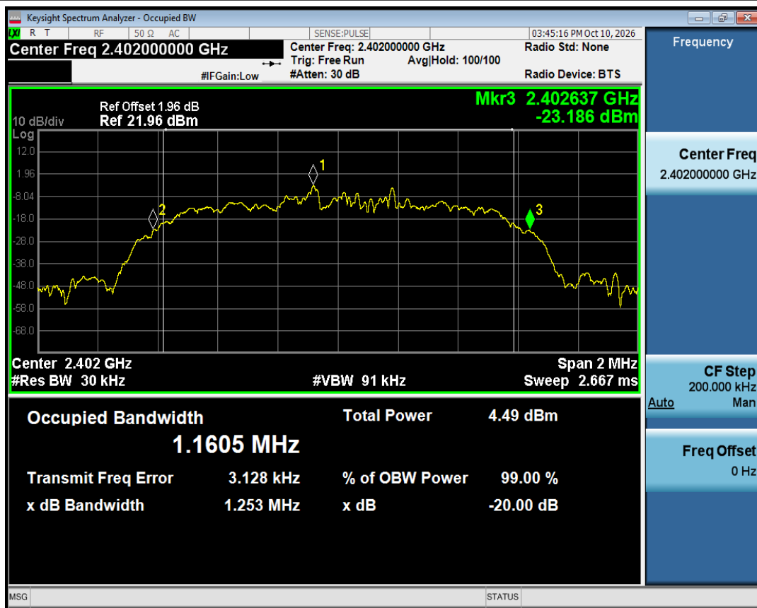
-20dB Bandwidth NVNT 2-DH5 2402MHz Ant1
