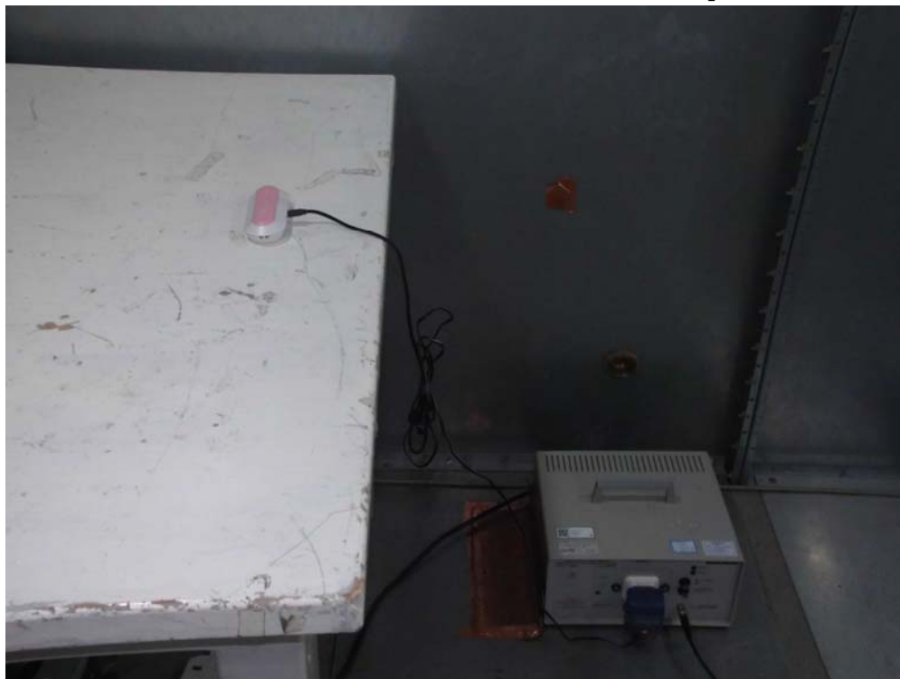
Measurement of Conducted Emission Test Set Up
