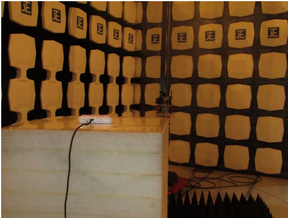
Measurement of Radiated Emission Test Set Up
