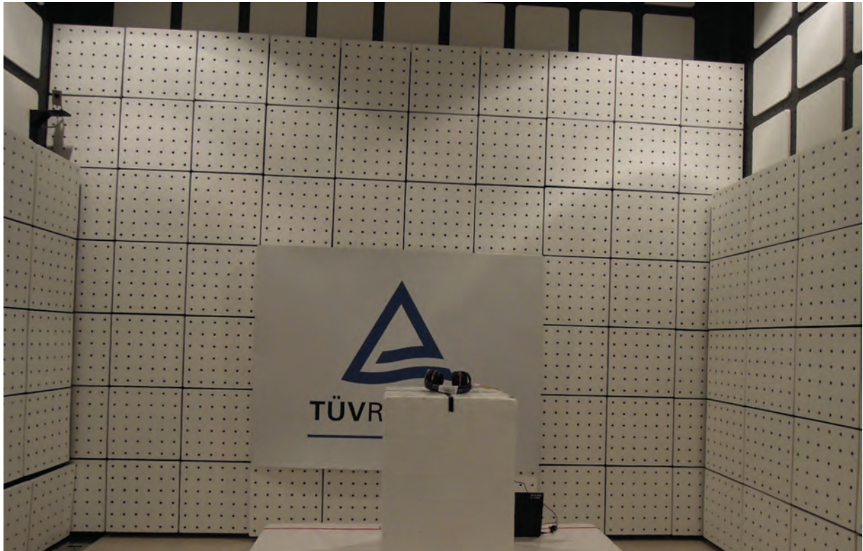
Photograph 1: Set-up for Spurious Emissions (Front View)
