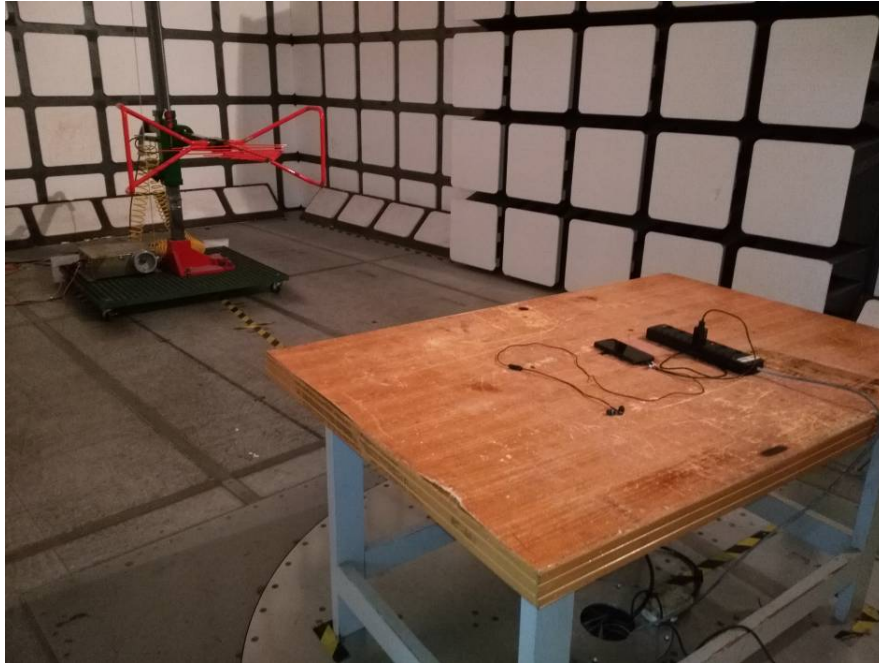
Radiated Emissions View (Below 1 GHz)
