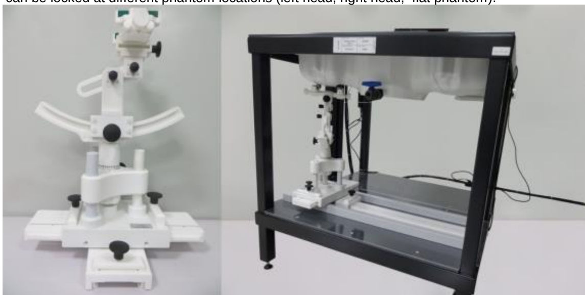
Device holder supplied by SATIMO
