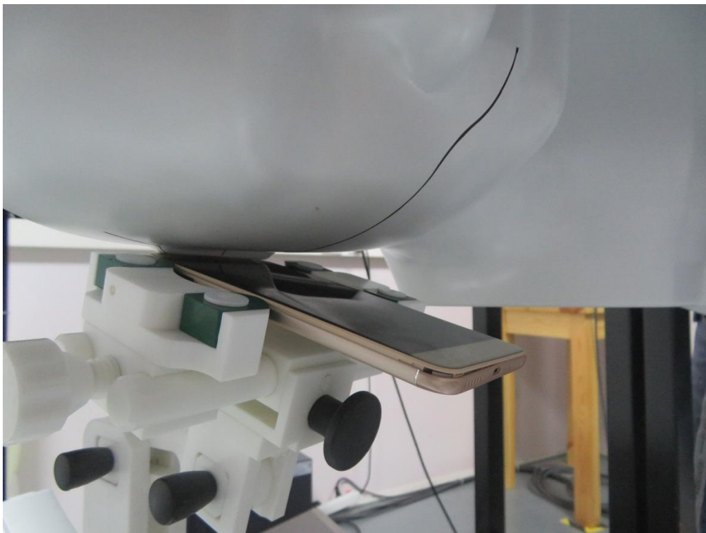
Head Setup Photo (Right Tilt)
