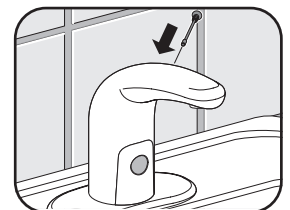
5. Install shut-off screw The temperature is now adjusted. Carefully test the new temperature. If necessary, adjust again.
