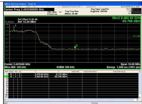
Out Of Band Emission(Right) 8DPSK_3-DH5_Channel Hopping
