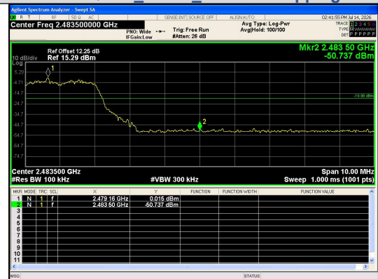
Out Of Band Emission(Right) \pi/4 DQPSK_2-DH5_Channel Hopping
