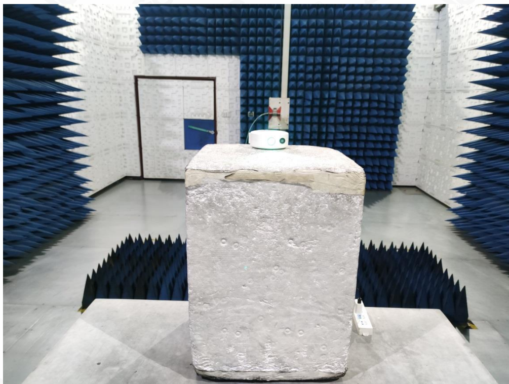
FCC RADIATED EMISSION TEST SETUP ABOVE 1GHZ
