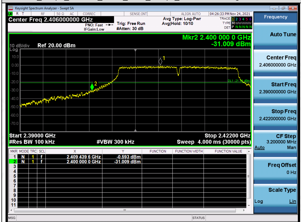
Test_Graph_802.11g_ANT1_2412_6Mbps_Lower Band Edge Emissions
