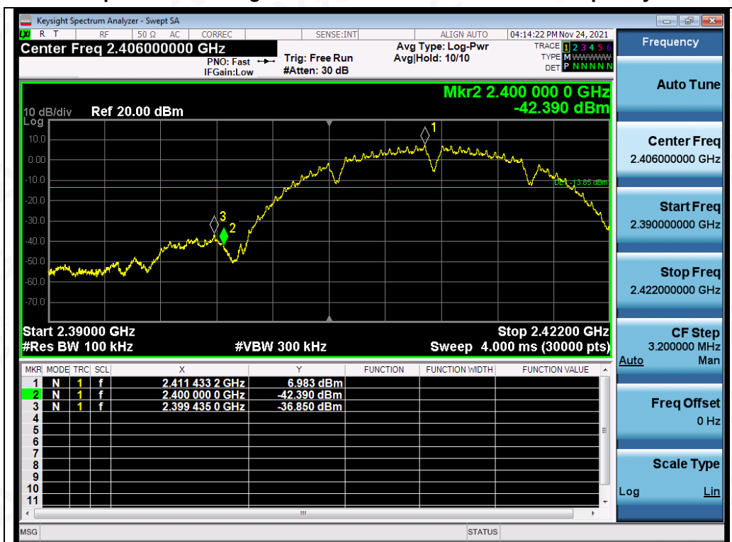
Test_Graph_802.11b_ANT1_2412_1Mbps_Lower Band Edge Emissions
