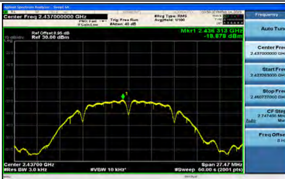
Maximum(average) power spectral density_11B_2462_Ant1
