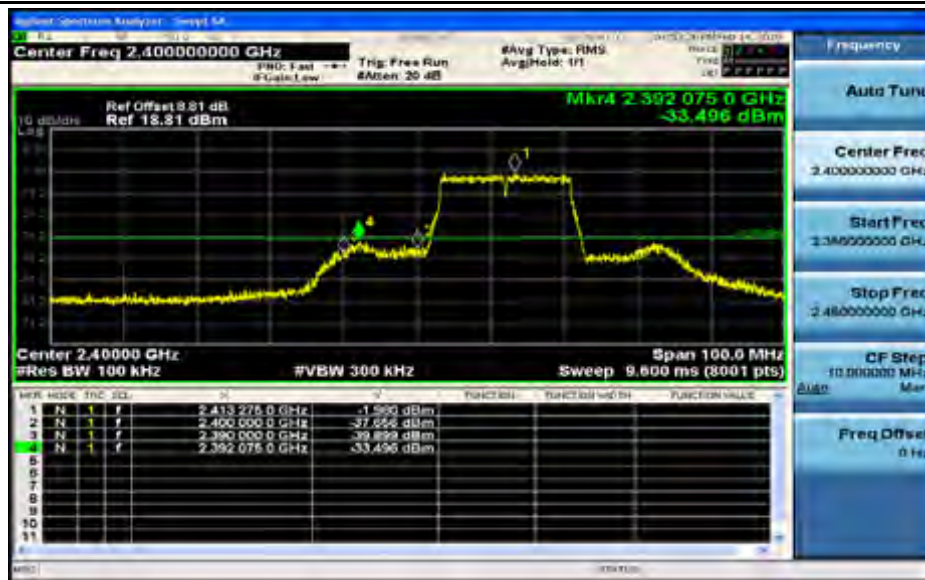
Band-edge for RF Conducted Emissions_11N20SISO_2462_Ant1
