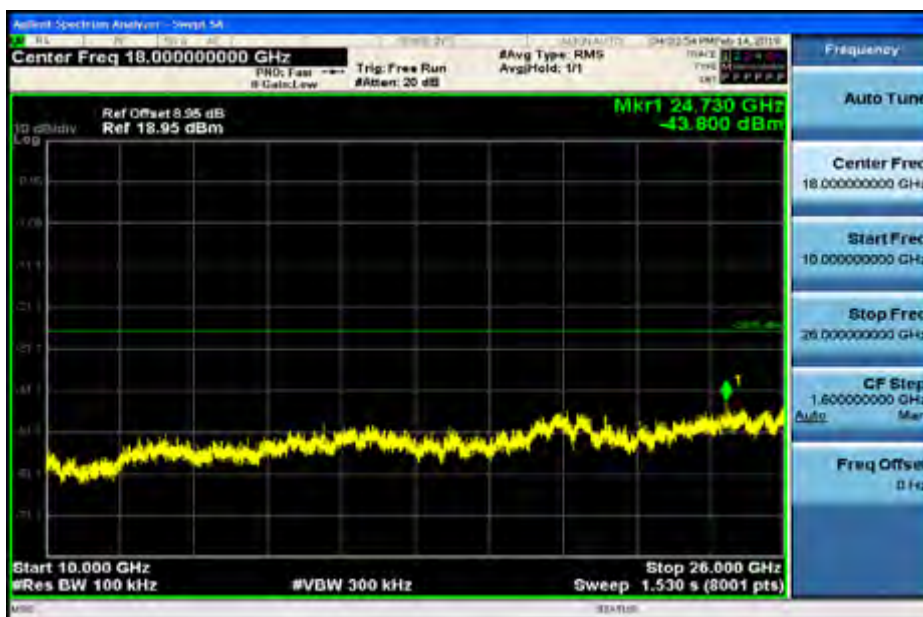
RF Conducted Spurious Emissions_11G_2412
