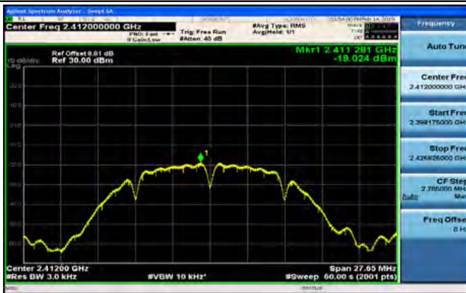
Maximum(average) power spectral density_11B_2437_Ant1
