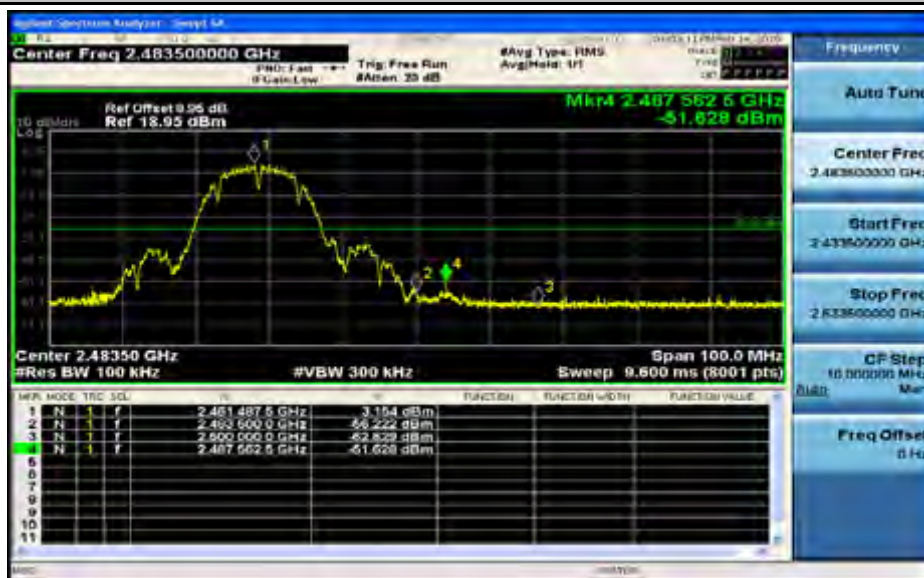
Band-edge for RF Conducted Emissions_11G_2412_Ant1
