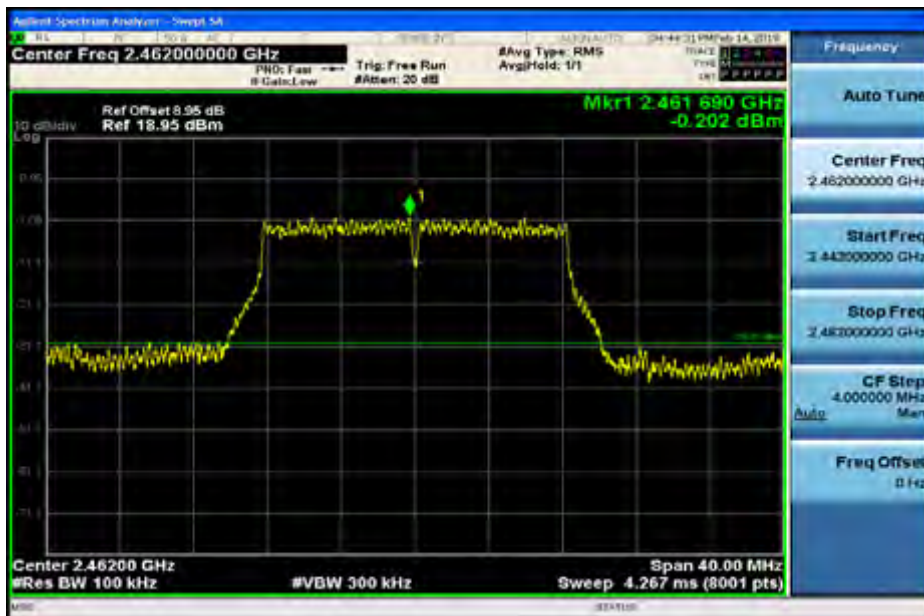
RF Conducted Spurious Emissions_11G_2462
