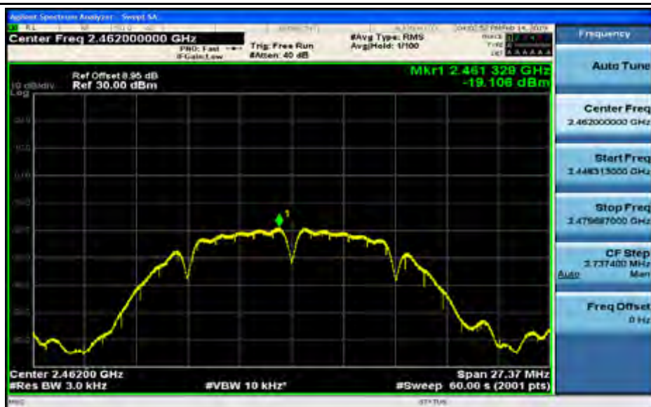
Maximum(average) power spectral density_11G_2412_Ant1
