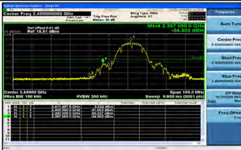
Band-edge for RF Conducted Emissions_11B_2462_Ant1
