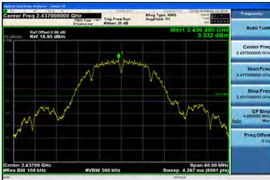
RF Conducted Spurious Emissions_11B_2437
