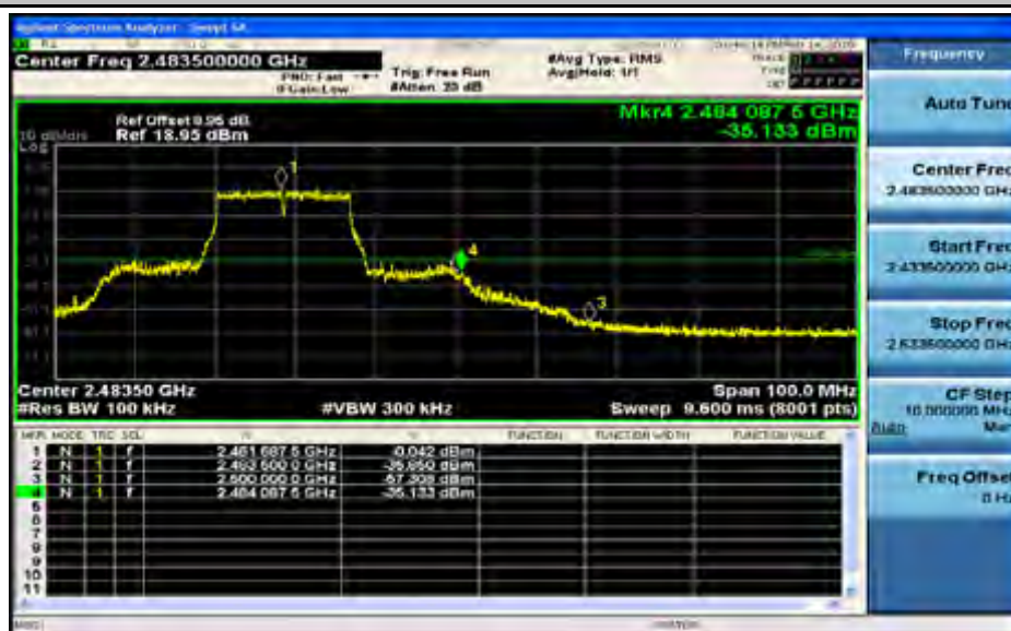
Band-edge for RF Conducted Emissions_11N20SISO_2412_Ant1
