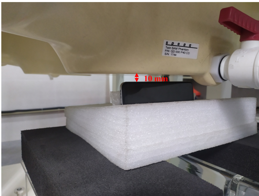
Body Left Setup Photo (10mm)
