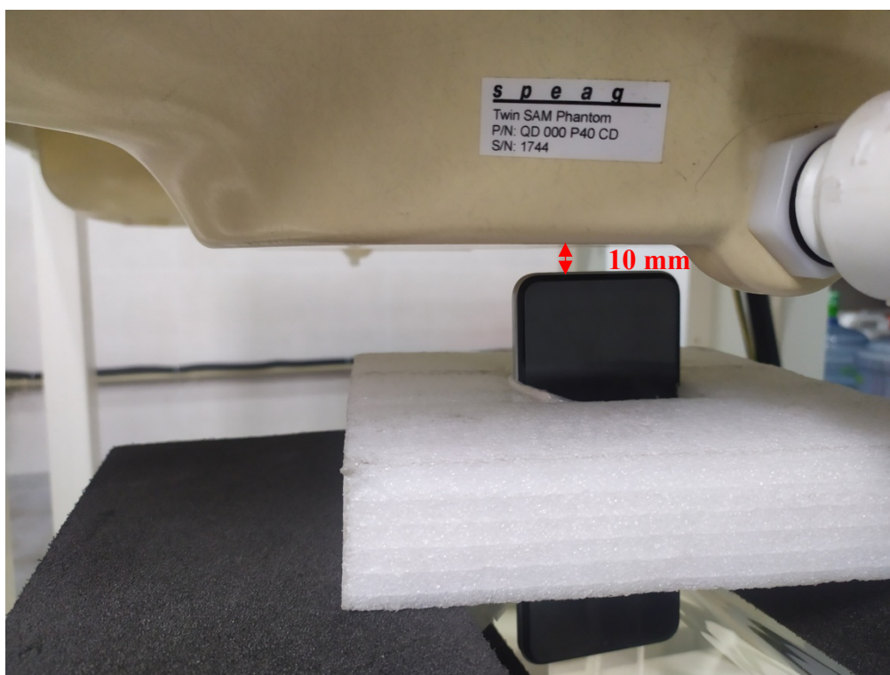
Body Bottom Setup Photo (10mm)
