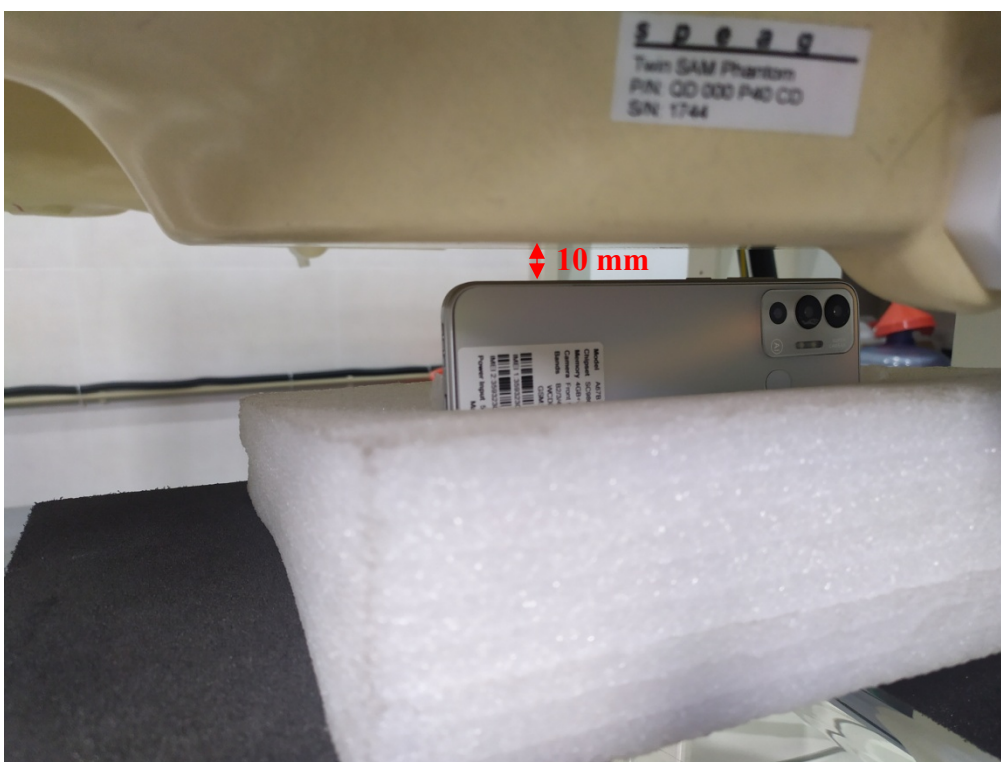
Body Right Setup Photo (10mm)
