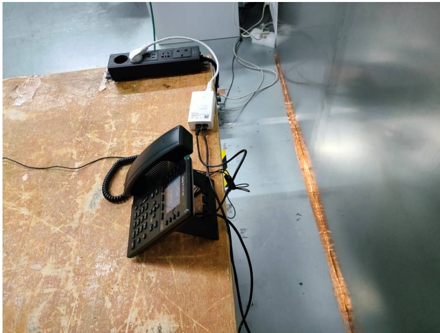
Conducted Emissions - Side View (Power by PoE)
