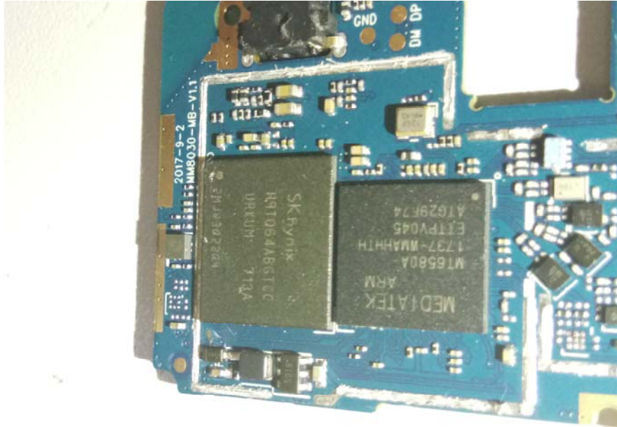
EUT – Main Chip 4 View
