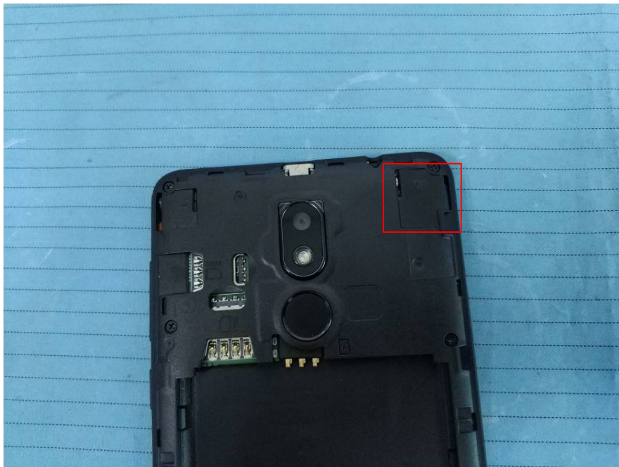
EUT –BT&WIFI Antenna View
