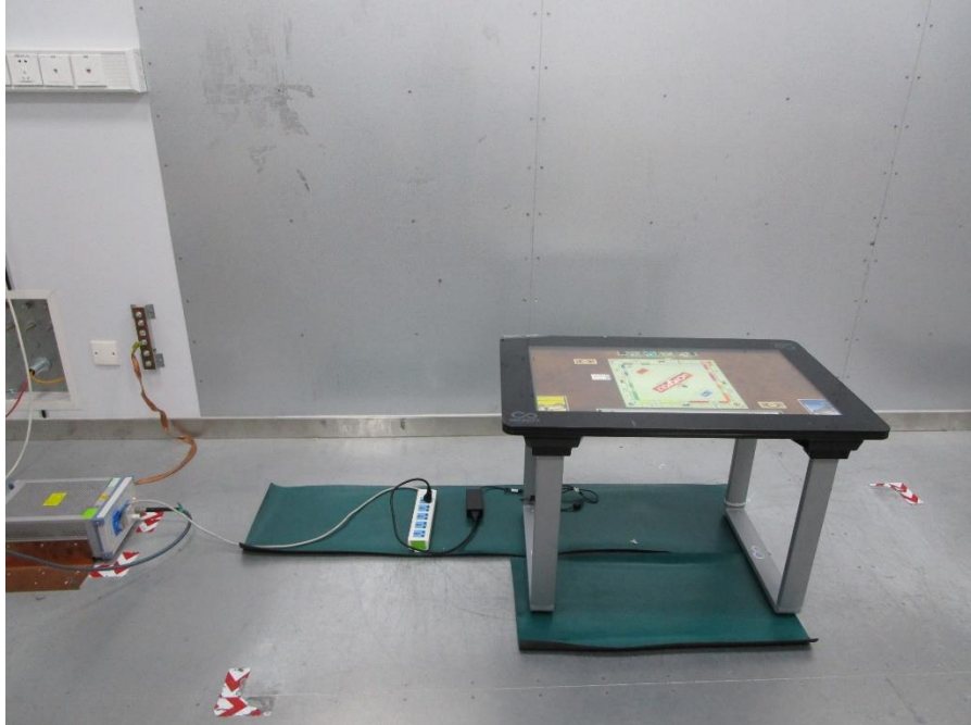
POWERLINE CONDUCTED EMISSIONS MEASUREMENT SETUP
