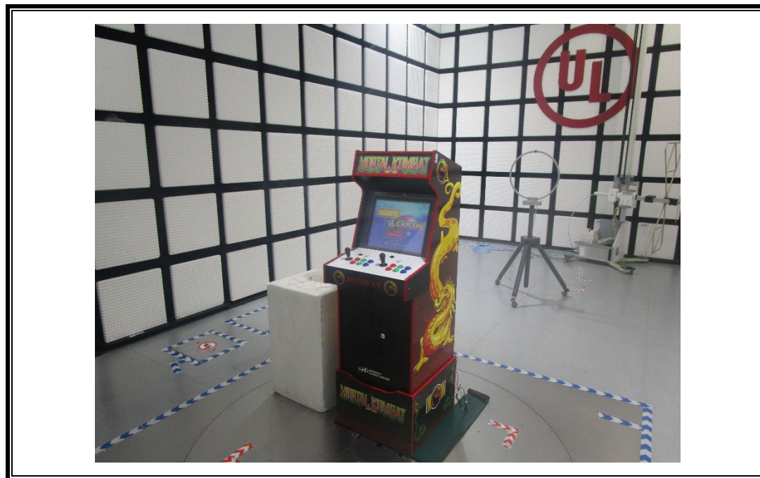
RADIATED RF MEASUREMENT SETUP (Below 30 MHz)
