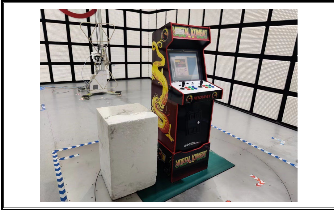
RADIATED RF MEASUREMENT SETUP (30 MHz ~ 1 GHz)
