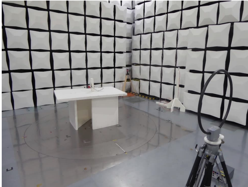
EUT Position #1 Test setup semi-anechoic chamber M276 Preliminary measurement
