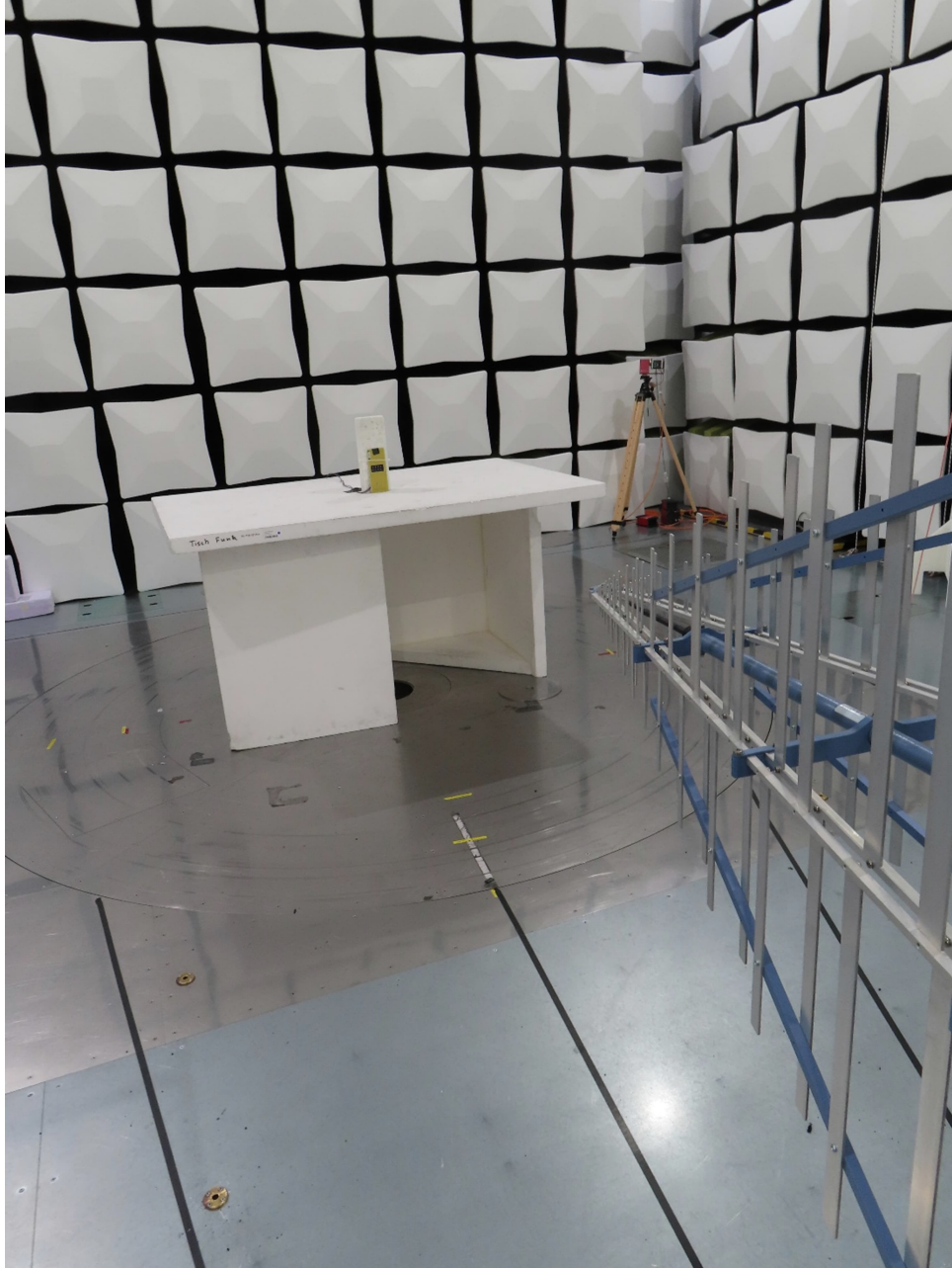
Test setup semi anechoic chamber M276, 30 MHz to 1 GHz
