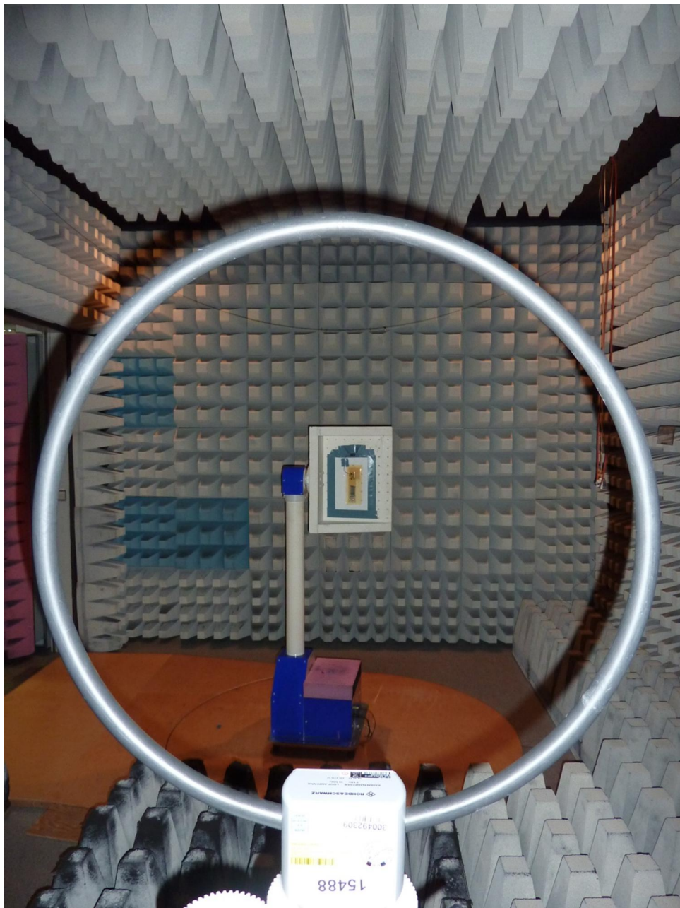
Test setup fully anechoic chamber 9 kHz – 30 MHz
