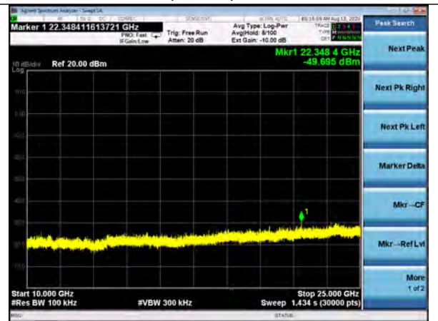
Conducted Spurious, 10-25GHz 802.11n, MCS7, Channel 11
