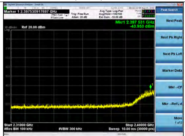
Conducted Spurious, 2310-2400MHz 802.11n, MCS7, Channel 1
