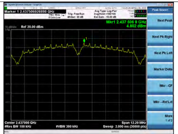
PSD, 802.11b, 1Mbps, Channel 6
