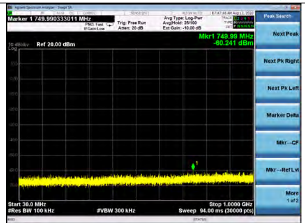
Conducted Spurious, 30-1000MHz 802.11b, 11Mbps, Channel 11
