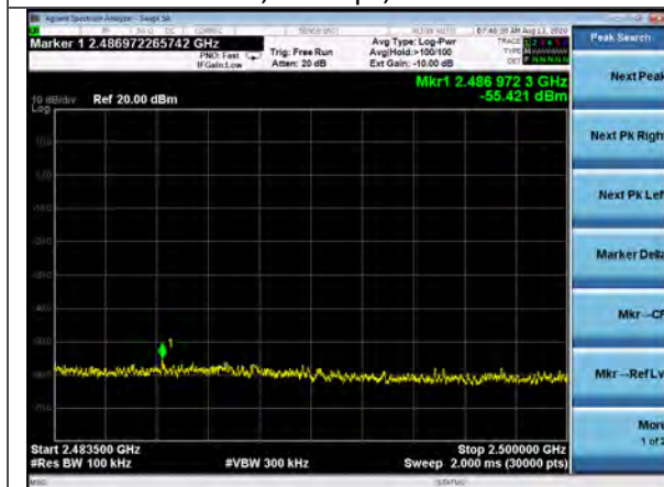
Conducted Spurious, 2483.5-2500MHz 802.11b, 11Mbps, Channel 11
