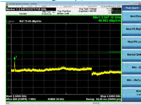
2.5-4 GHz, Vertical Antenna, Vertical EUT 802.11b, 1Mbps, Channel 11
