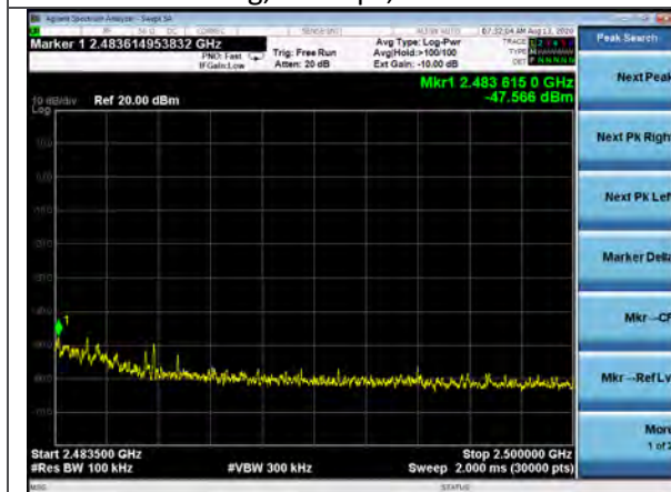
Conducted Spurious, 2483.5-2500MHz 802.11g, 54Mbps, Channel 11
