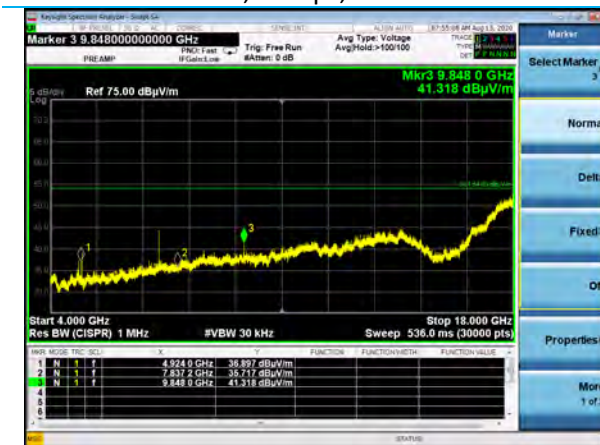
4-18 GHz, Vertical Antenna, Side EUT 802.11b, 1Mbps, Low Channel
