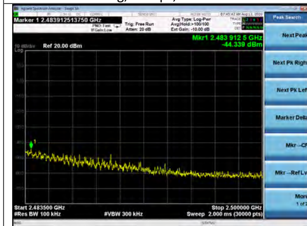
Conducted Spurious, 2483.5-2500MHz 802.11g, 6Mbps, Channel 11
