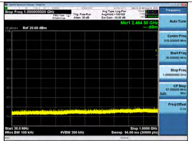
Conducted Spurious, 30-1000MHz 802.11n, MCS7, Channel 11
