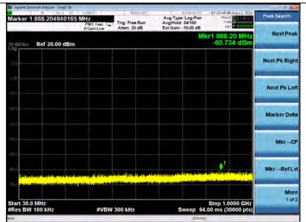
Conducted Spurious, 30-1000MHz 802.11n, MCS0, Channel 11
