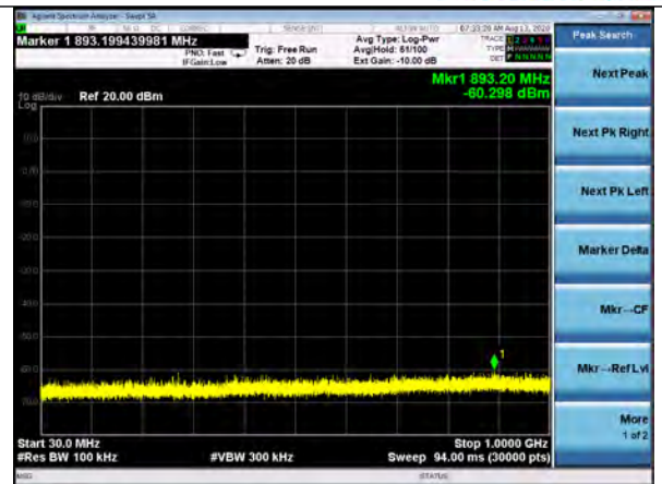
Conducted Spurious, 30-1000MHz 802.11g, 54Mbps, Channel 11
