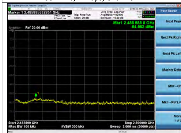
Conducted Spurious, 2483.5-2500MHz 802.11b, 1Mbps, Channel 11
