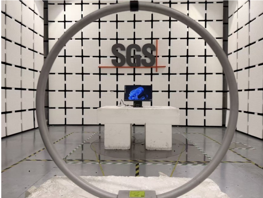
Radiated Test (9kHz-30MHz)
