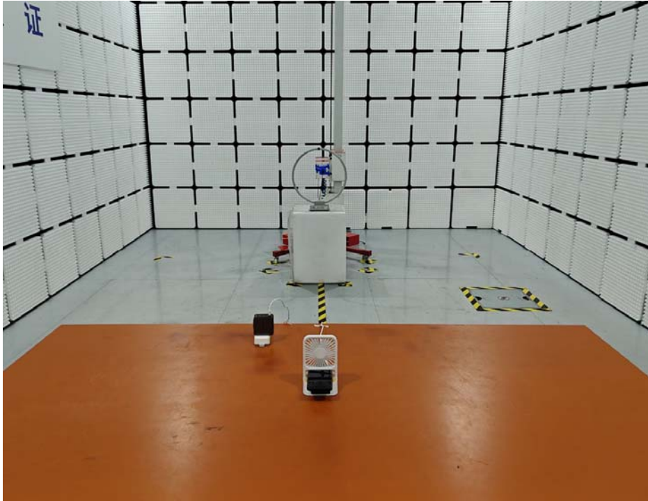
Radiated Emission Above 30MHz
