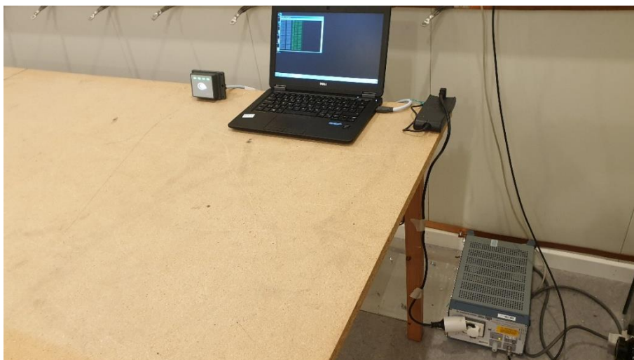
Photo 9. AC Conducted emission test set up.
