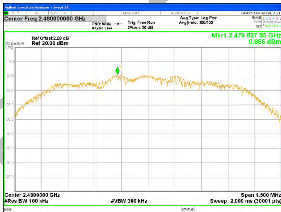
Tx. Spurious NVNT 2-DH1 2480MHz Ant1 Emission
