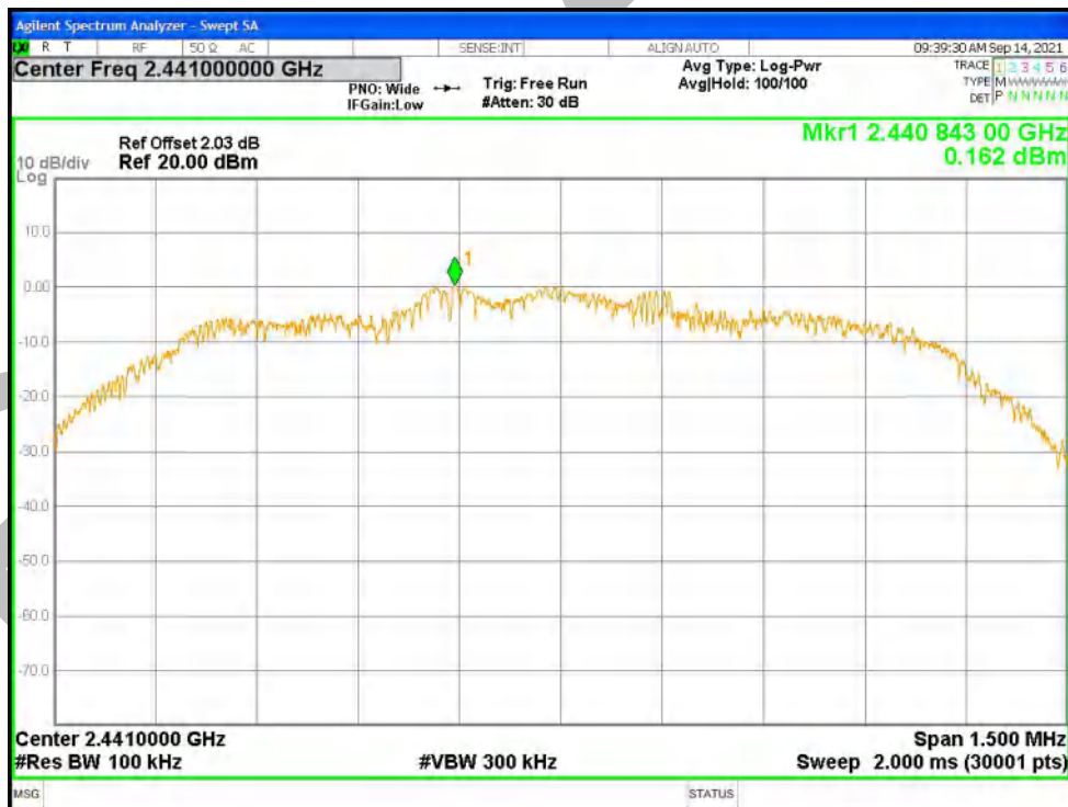
Tx. Spurious NVNT 2-DH1 2441MHz Ant1 Emission
