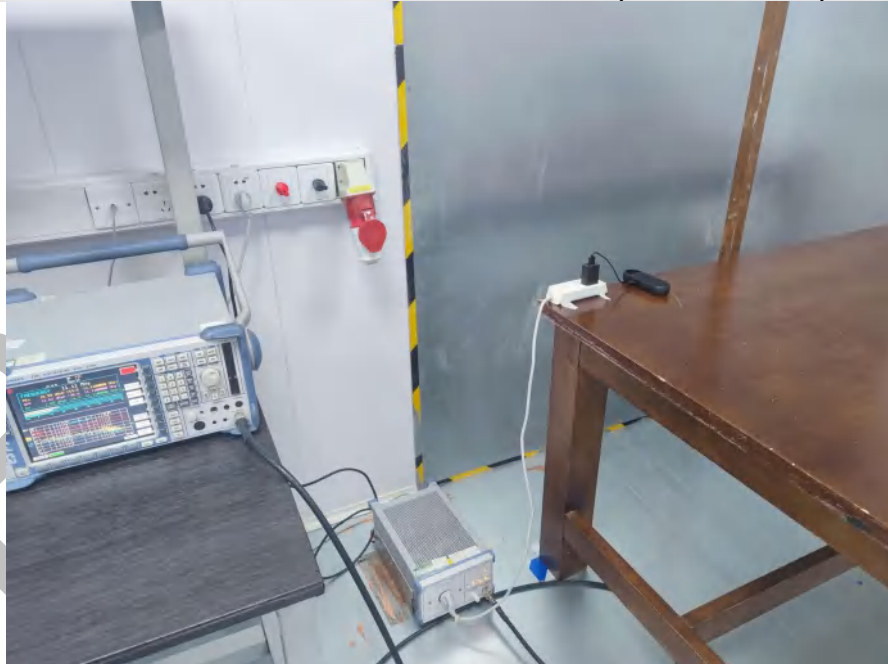
Conducted Emissions at AC Power Line (150kHz-30MHz)
