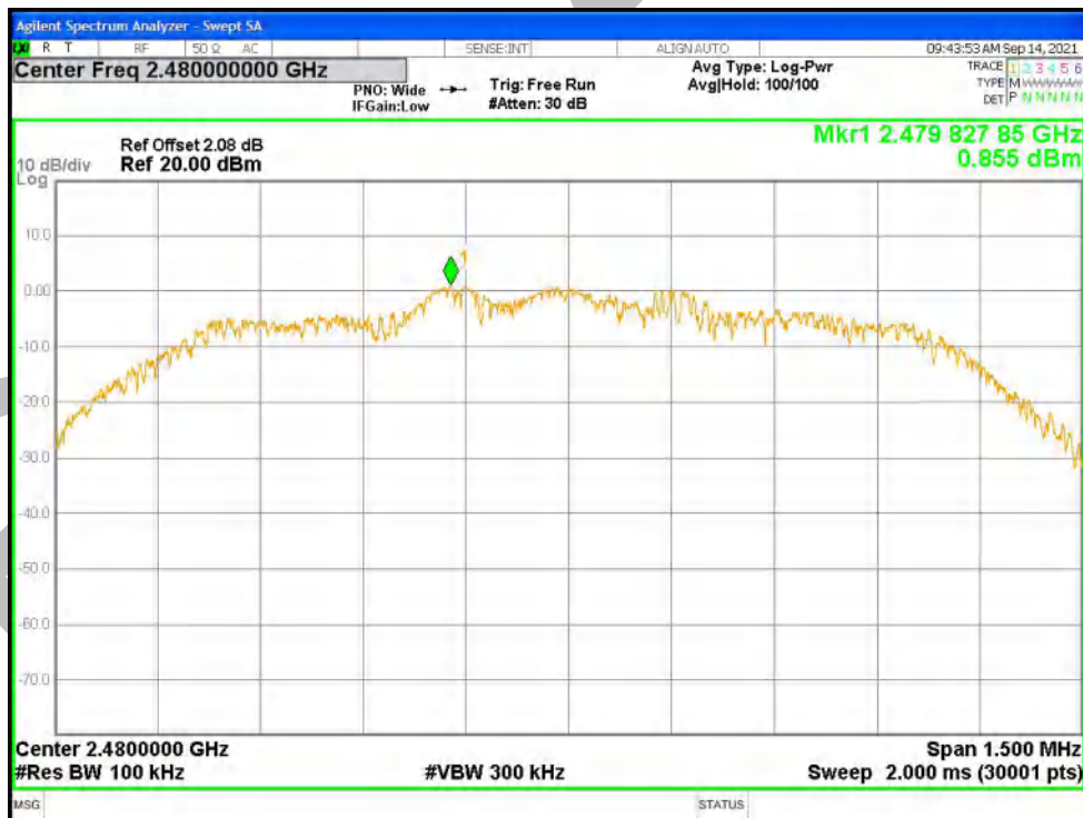
Tx. Spurious NVNT 2-DH1 2480MHz Ant1 Emission
