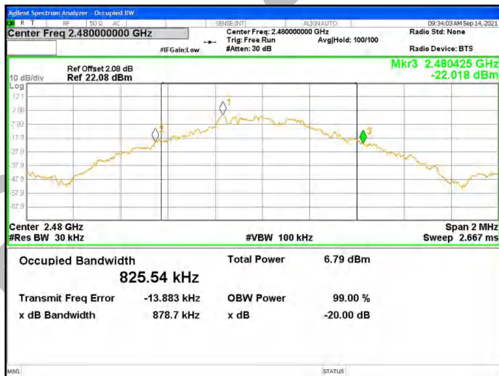
-20dB Bandwidth NVNT 2-DH1 2402MHz Ant1
