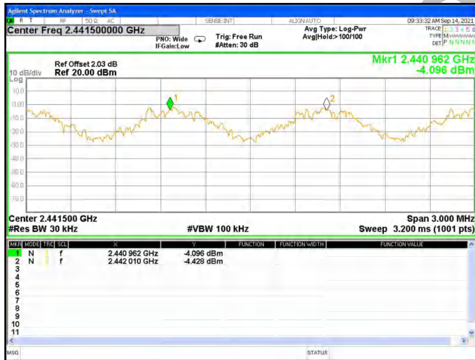
CFS NVNT 2-DH1 2441MHz Ant1
