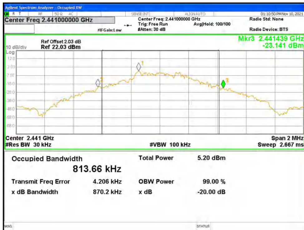
-20dB Bandwidth NVNT 1-DH1 2480MHz Ant1
