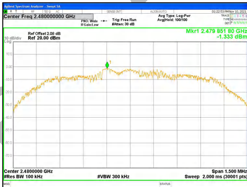
Tx. Spurious NVNT 2-DH1 2480MHz Ant1 Emission
