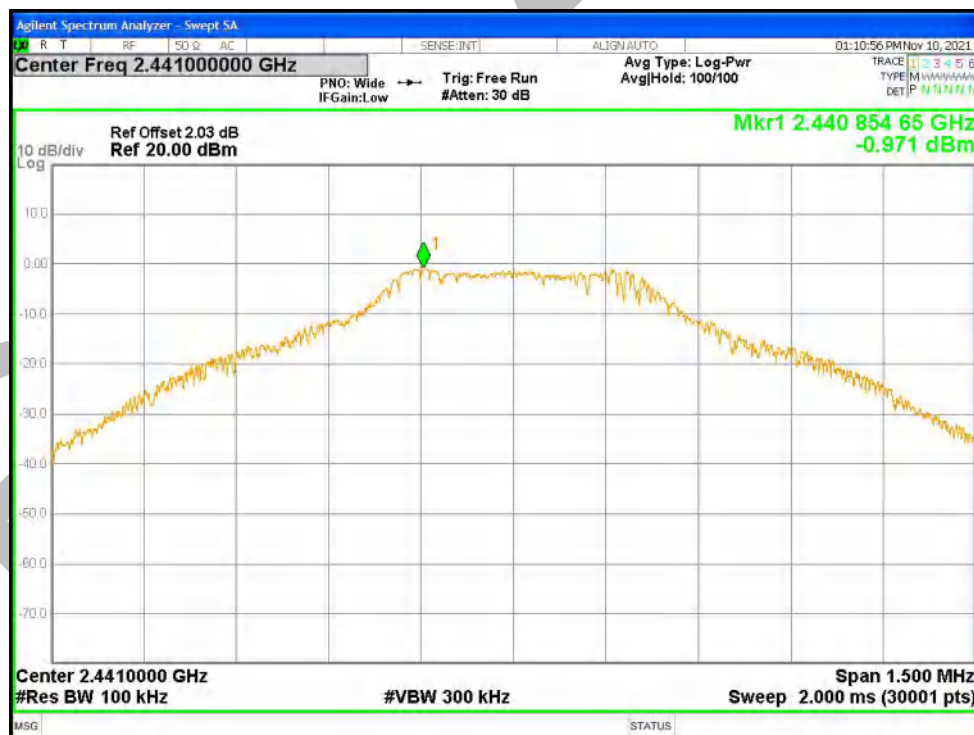
Tx. Spurious NVNT 1-DH1 2441MHz Ant1 Emission
