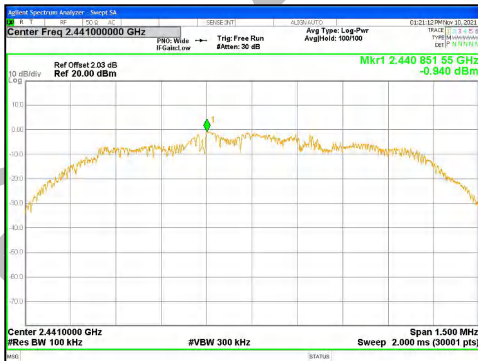
Tx. Spurious NVNT 2-DH1 2441MHz Ant1 Emission
