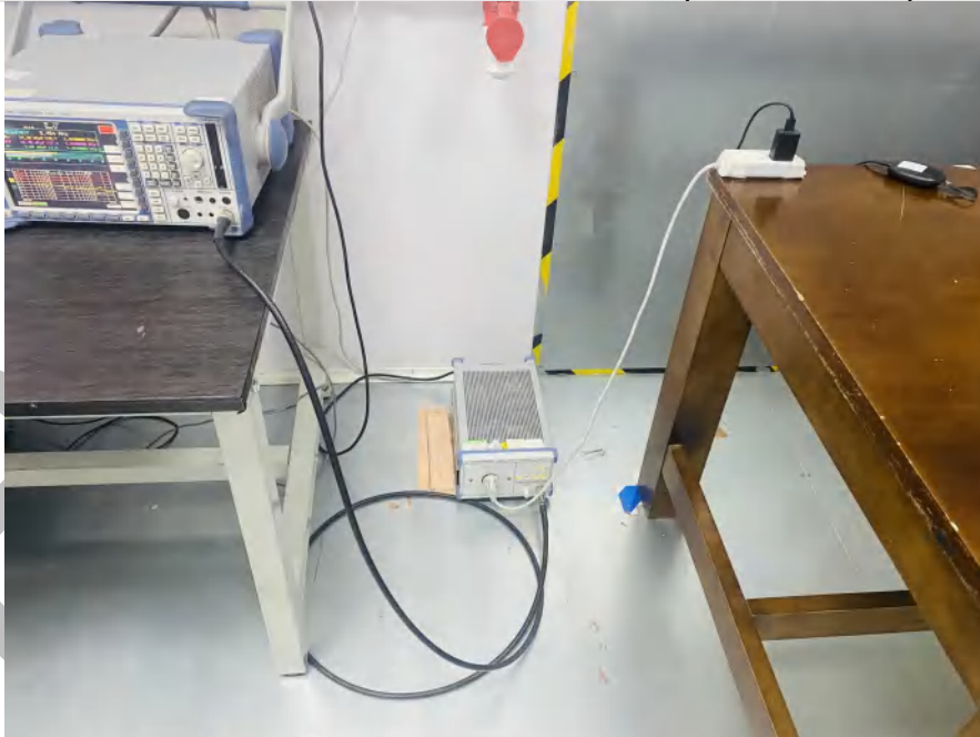
Conducted Emissions at AC Power Line (150kHz-30MHz)
