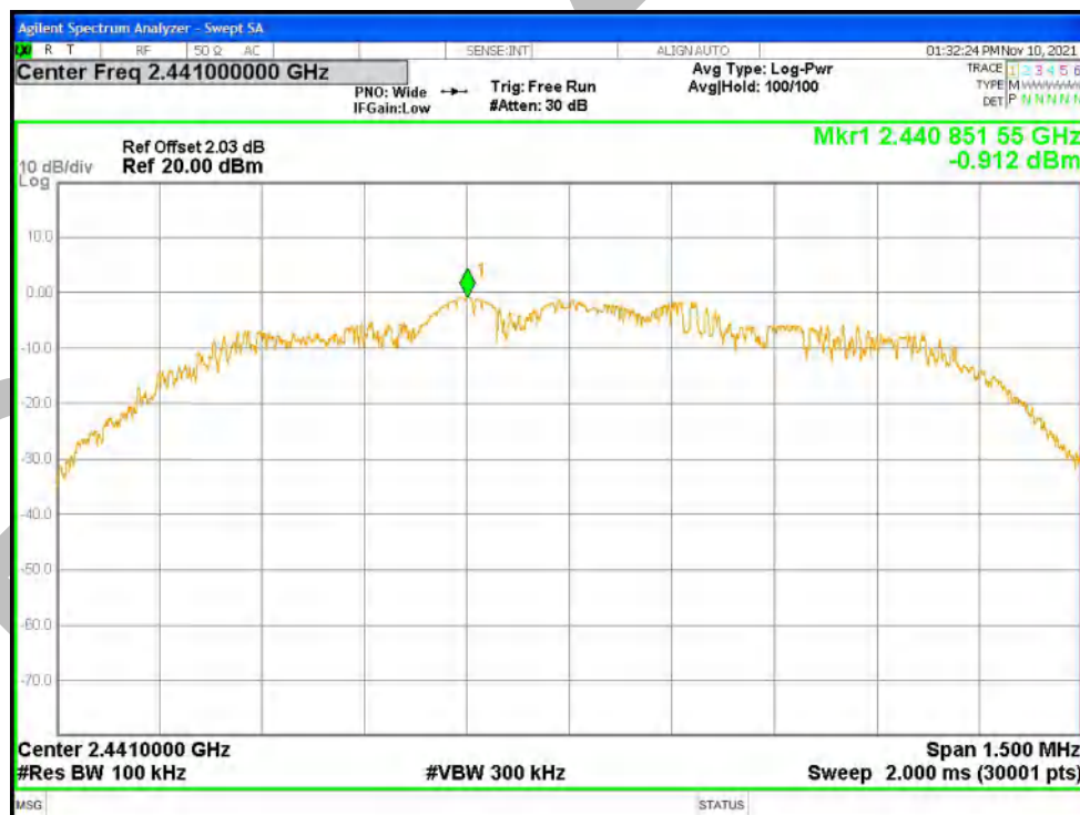
Tx. Spurious NVNT 3-DH1 2441MHz Ant1 Emission
