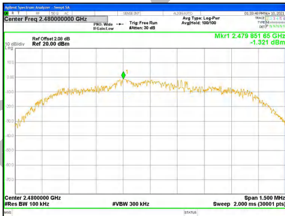
Tx. Spurious NVNT 3-DH1 2480MHz Ant1 Emission
