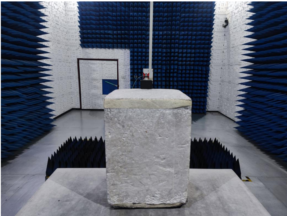
RADIATED EMISSION TEST SETUP ABOVE 1GHz
