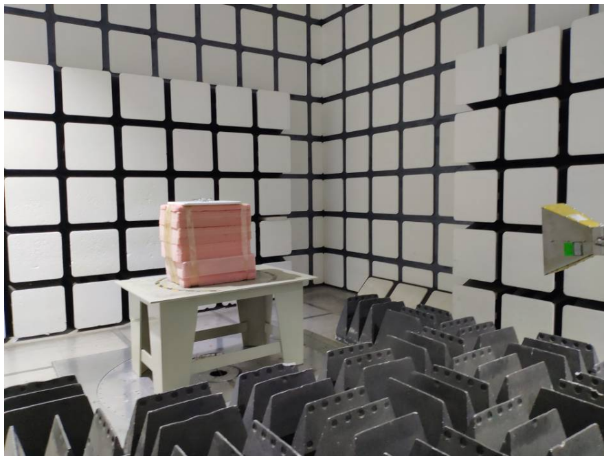
Radiated Emissions View (Above 1 GHz)
