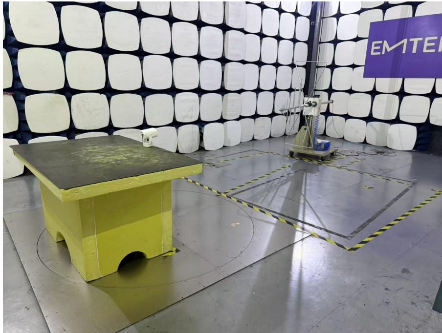
Spurious Emission Test Setup (Above 1GHz)
