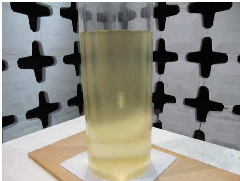
Radiated emissions test set inside human body simulator. General view
