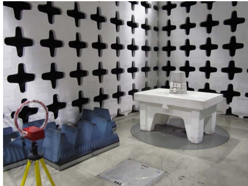
Radiated emissions test set up below 30MHz
