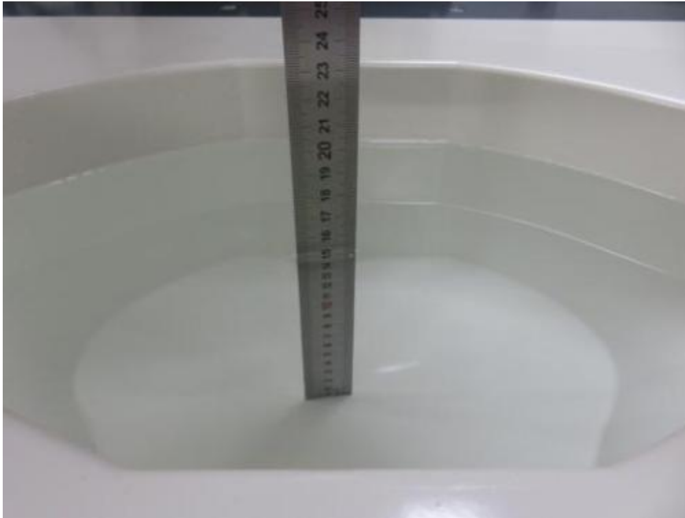
Photograph of the depth in the Body Phantom (2450MHz, 15.6cm depth)
