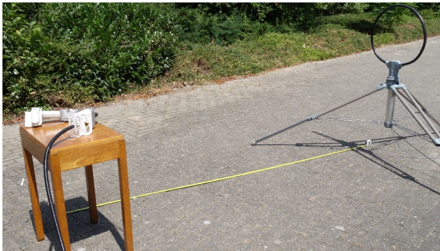
Radiated emissions test setup below 30 MHz
