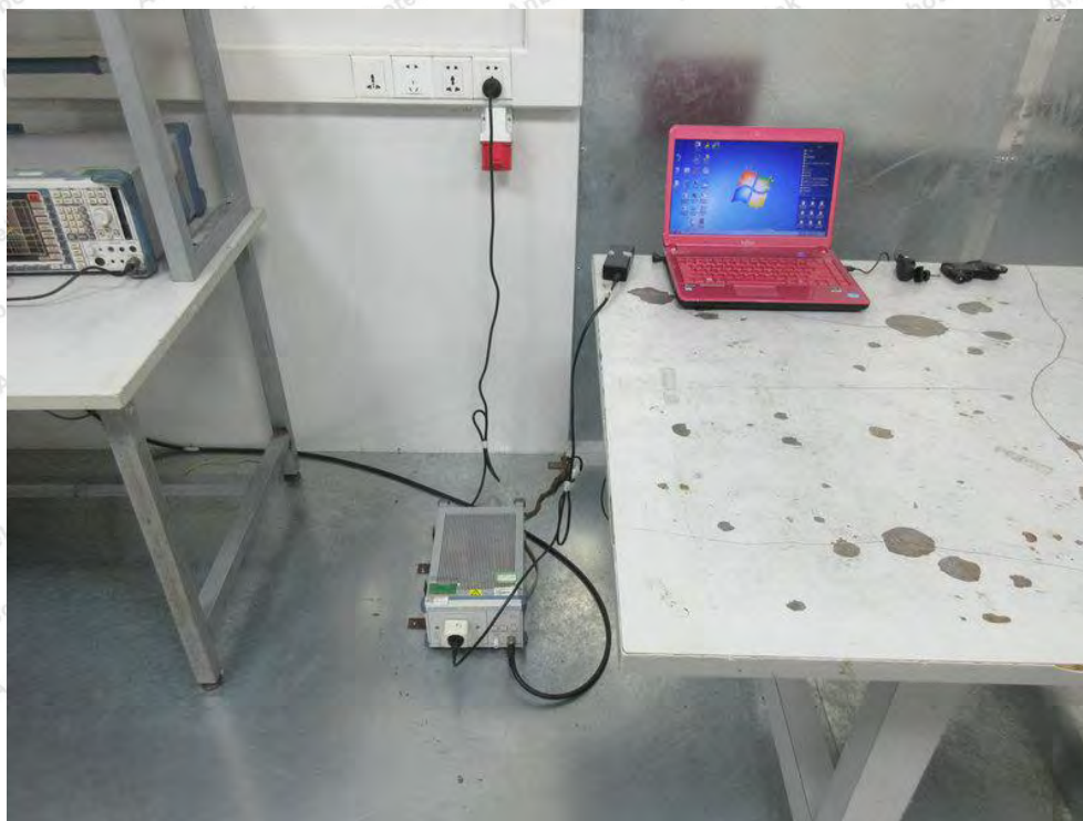
Photo of Power Line Conducted Emission Test
