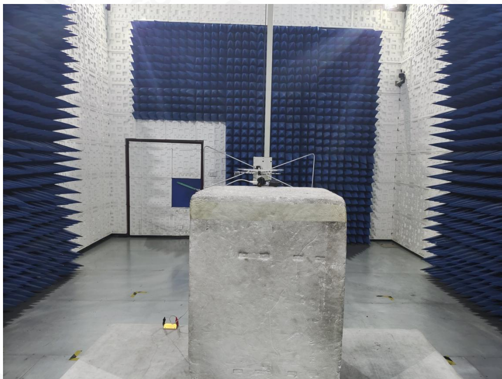
RADIATED EMISSION TEST SETUP ABOVE 1G
