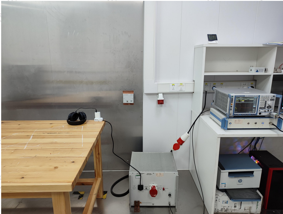
Photo of Conducted Emission Measurement
