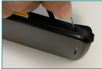
Figure 2-2 Insert the small hole with a metal pin
