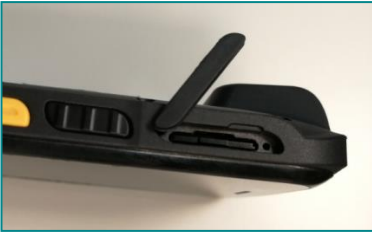
Figure 2-1 Pull out the plug
