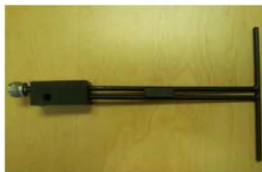
Figure 1 – MVG COMOSAR Validation Dipole
