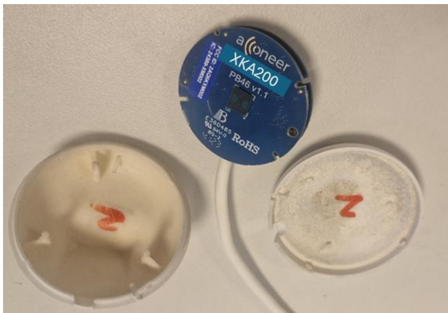
Figure 5, The XKA200+BA connector board connected with front and backside plastic housing.
