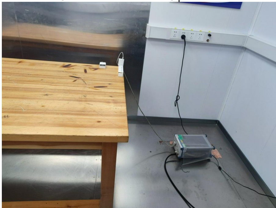
Conducted Emission at AC power line
