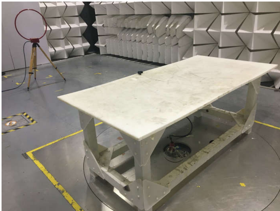
Radiated spurious emission Test Setup-1(Below 30MHz)
