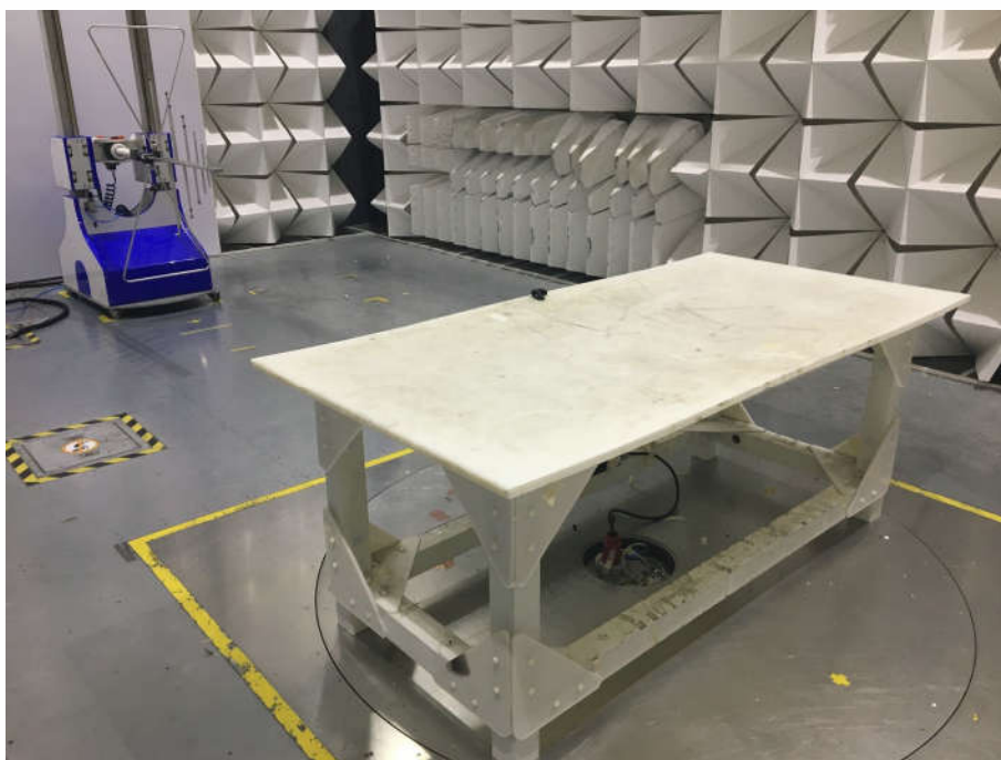
Radiated spurious emission Test Setup-2(Below 1GHz)
