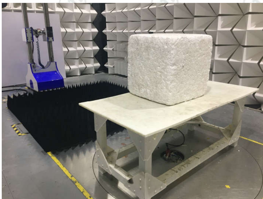
Radiated spurious emission Test Setup-4(Above 1GHz)
