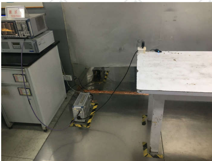
Conducted Emissions Test Setup
