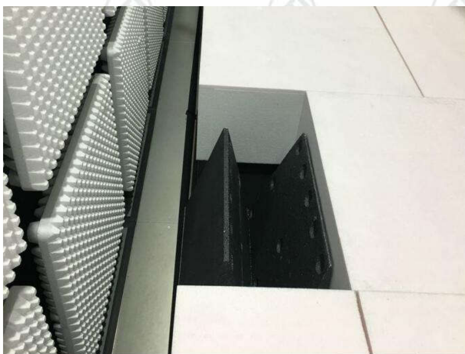
Radiated spurious emission Test Setup-4(Above 1GHz) There are absorbing materials under the ground.
