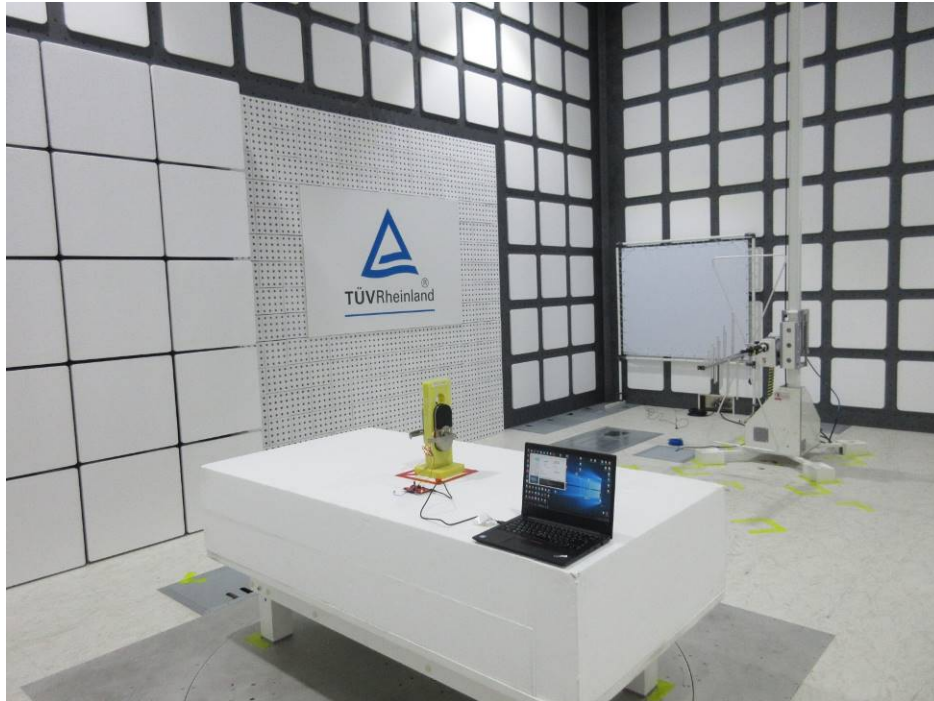
Photograph 3: Set-up for Spurious Emissions (Back View 1)
