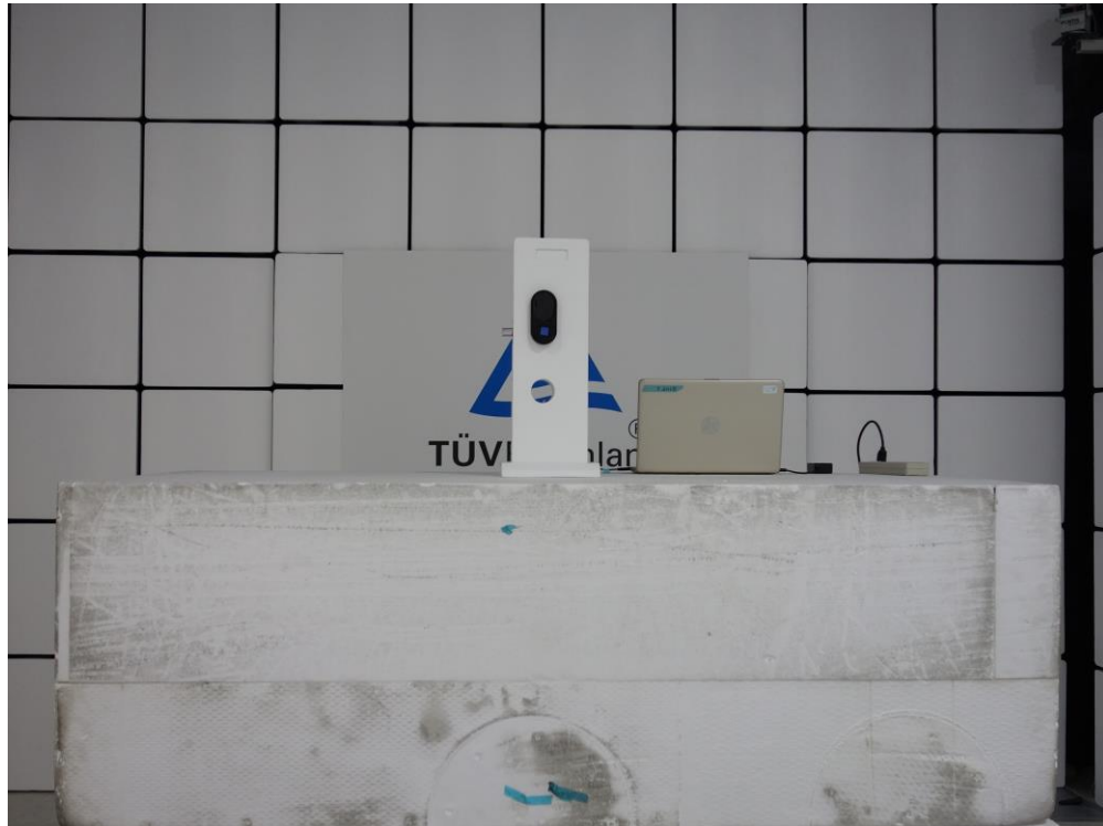
Photograph 1: Set-up for Spurious Emissions (Front View 1)
