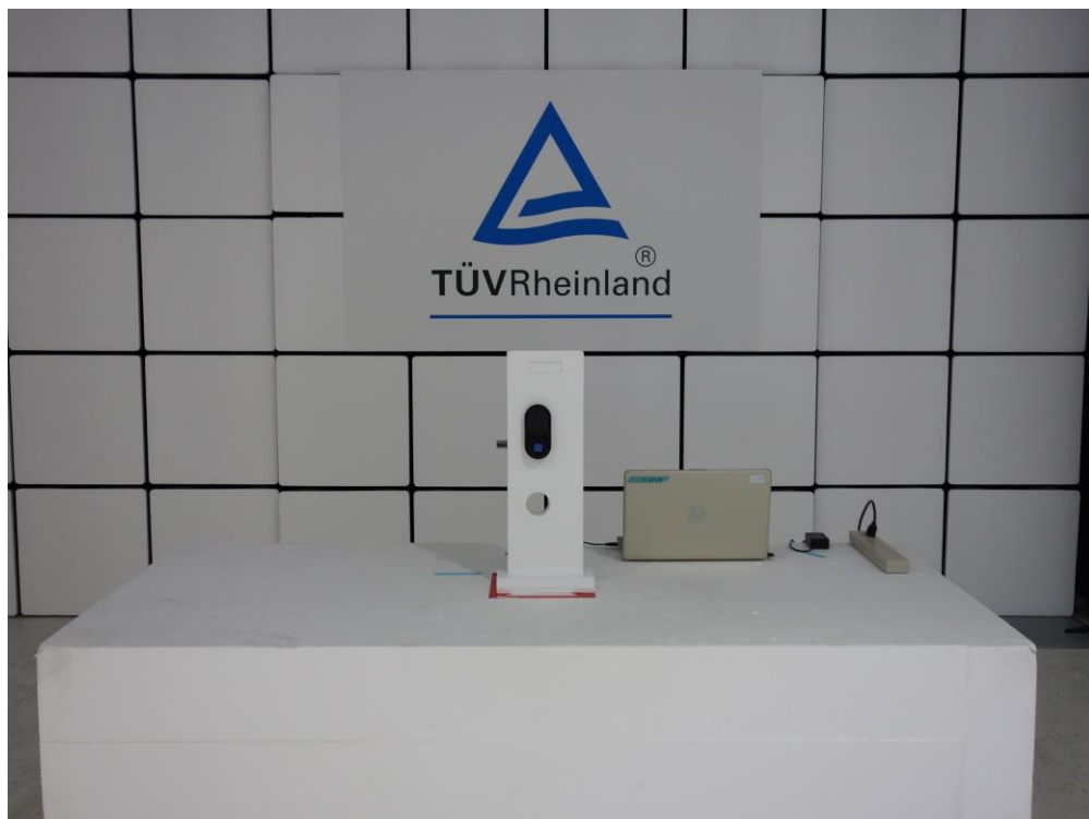
Photograph 2: Set-up for Spurious Emissions (Front View 2)
