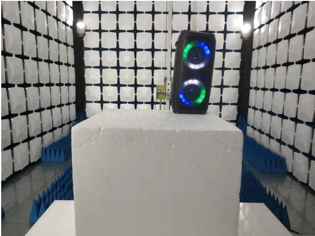
Below 1GHz for radiated emission test setup
