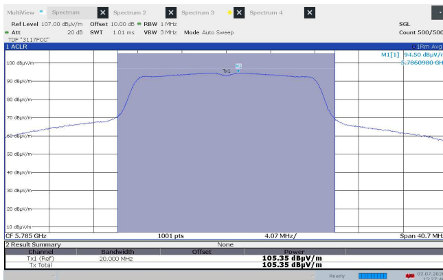
EIRP, 5785 MHz, 802.11a, 6Mb, EUT V, Ant 1, VP, Max
