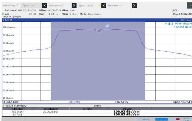
EIRP, 5560 MHz, 802.11a, 6Mb, EUT V, Ant 1, VP, Max
