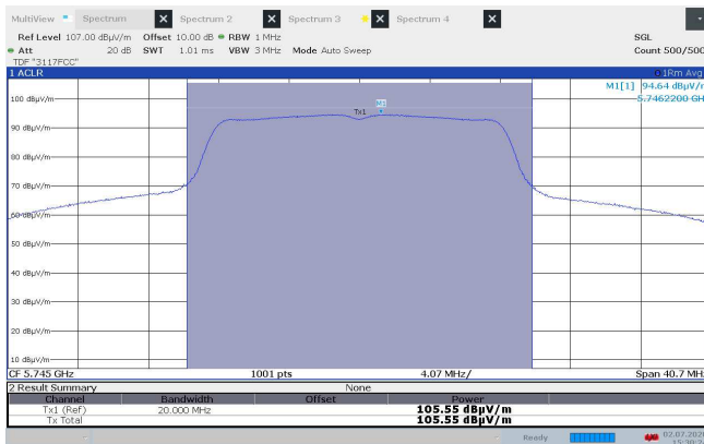
EIRP, 5745 MHz, 802.11a, 6Mb, EUT V, Ant 1, VP, Max
