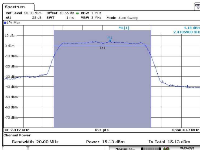
Peak Conducted Power, 2412 MHz, 802.11g, 6Mb
